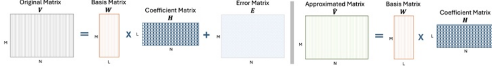
Figure 1: Formulation of Nonnegative Matrix Factorization (NMF)
